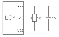
$V_{DD}$ ~ $V_0$ : LCD Driving voltage VR: 10k~20k
