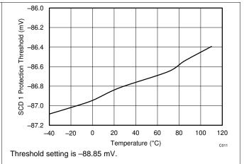
Figure 12. Short Circuit Discharge 1 Protection Threshold vs. Temperature
