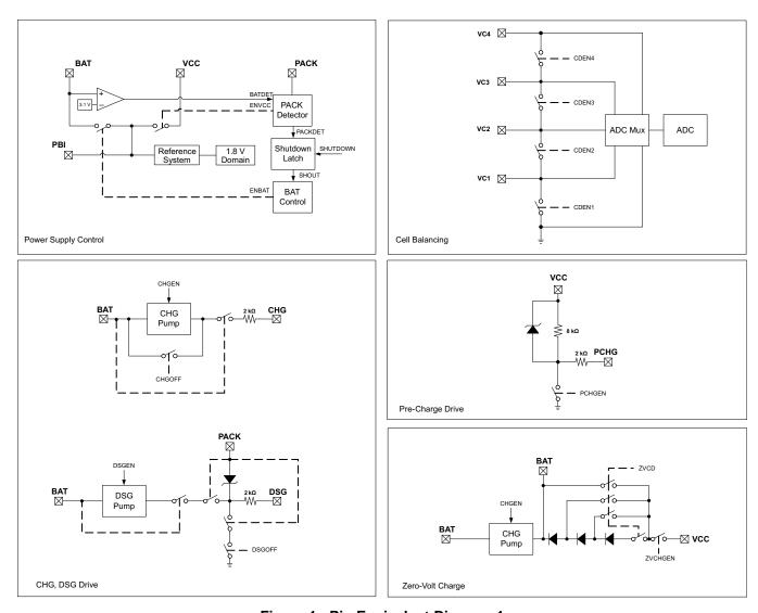
Figure 1. Pin Equivalent Diagram 1
