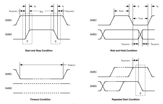
Figure 4. SMBus Timing Diagram
