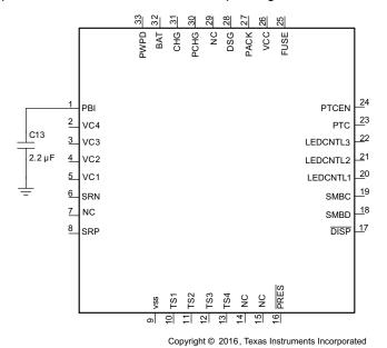
Figure 27. Power Supply Decoupling
