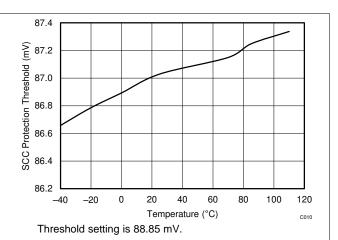
Figure 38. Short Circuit Charge Protection Threshold Vs.
