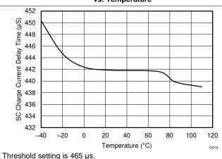
Figure 15. Short Circuit Charge Current Delay Time vs.
