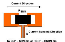
Figure 45. Sensing Resistor PCB Layout
