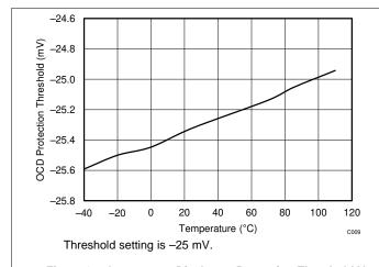
Figure 37. Overcurrent Discharge Protection Threshold Vs.
