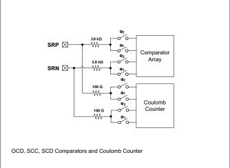
Figure 3. Pin Equivalent Diagram 3
