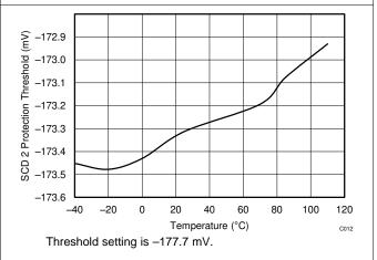
Figure 40. Short Circuit Discharge 2 Protection Threshold Vs. Temperature
