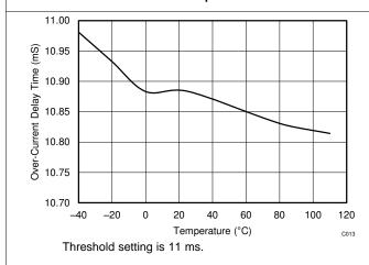
Figure 41. Overcurrent Delay Time Vs. Temperature
