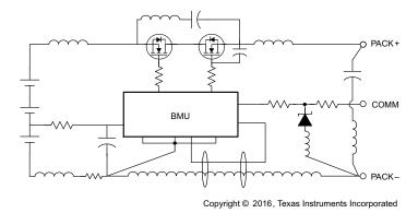
Figure 44. Avoid Close Spacing Between High-Current and Low-Level Signal Lines
