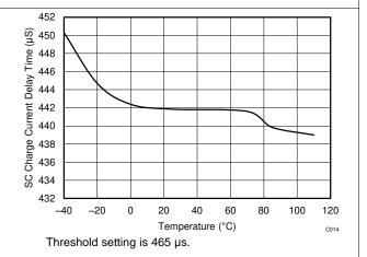
Figure 42. Short Circuit Charge Current Delay Time Vs.
