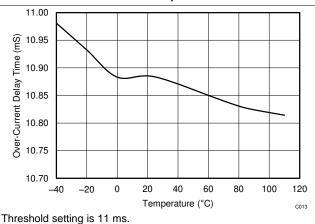
Figure 14. Overcurrent Delay Time vs. Temperature
