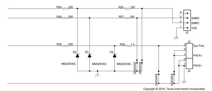
Figure 30. ESD Protection for SMB Communication
