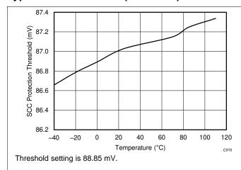
Figure 11. Short Circuit Charge Protection Threshold vs. Temperature
