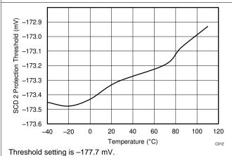
Figure 13. Short Circuit Discharge 2 Protection Threshold vs. Temperature
