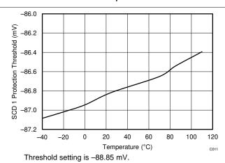
Figure 39. Short Circuit Discharge 1 Protection Threshold Vs. Temperature
