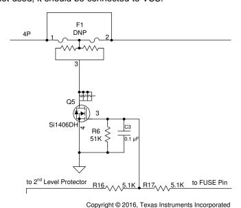
Figure 31. FUSE Circuit
