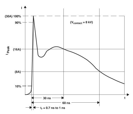
Figure 10. Typical Current Waveform of IEC61000-4-2 ESD Generator
