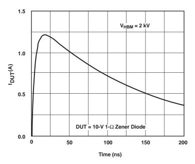
Figure 8. Typical HBM Current Waveform
