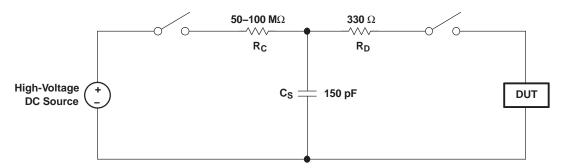
Figure 9. Simplified IEC61000-4-2 ESD Test Circuit
