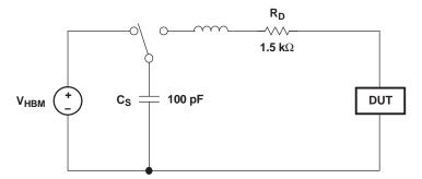
Figure 7. HBM ESD Test Circuit
