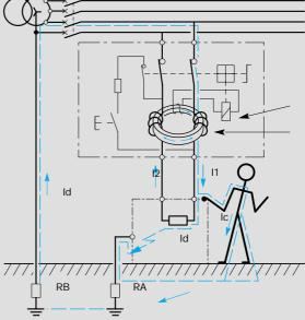
Current flowing through torroid in healthy circuit
