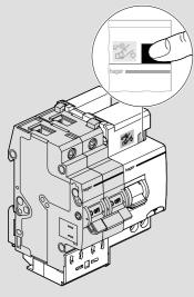
By pushing the "lock" button it will bolt both devices together mechanically, thus forbidding a dismantling of the products without deteriorating the RCCB add-on block (compliance to annex G of standard EN 61-009).
