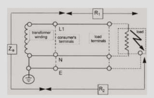
Components of earth fault loop impedance  $(Z_S)$  in a system. (Earth fault at load between conductor and casing).
