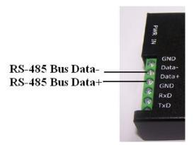
1. Connect the data cable to the Data+1~4, Data-1~4 in downstream ports of SER-4485-SI-M for four RS-485 bus or devices.
