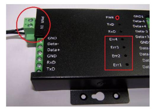
The SER-4485-SI-M power input is designed with a diode bridge circuit. You don't need to care the input DC power polarity, and you can also use an AC to AC 9V ~ 48V power adapter for SER-4485-SI-M.
