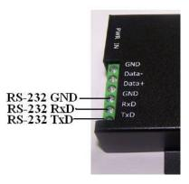
• For converting RS-485 to RS-485 hub, connect the data cable to the Data+, Datain upstream ports of SER-4485-SI-M. You need to connect the Data+ pin to the Data+ signal of an external RS-485 bus and the Data- pin to the Data- signal of an external RS-485 bus.
