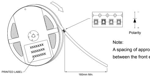
A spacing of approximately 160mm between the front edge of tape
