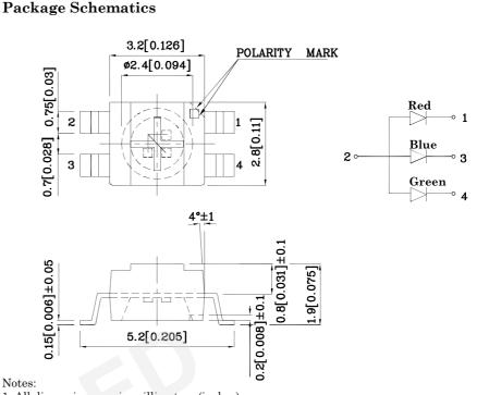
1. All dimensions are in millimeters (inches). 2. Tolerance is  $\pm 0.2(0.008")$  unless otherwise noted. 3. Specifications are subject to change without notice.
