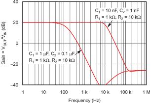
Figure 30. OPA348 Two-Pole, Low-Pass Sallen-Key AC Gain vs Frequency Response
