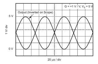
Figure 24. OPA348 Features Rail-to-Rail Input and Output
