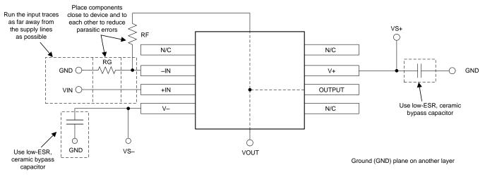
Figure 31. Operational Amplifier Board Layout for Noninverting Configuration
