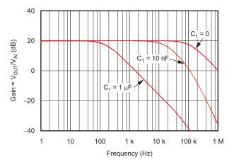
Figure 28. OPA348 Single-Pole AC Gain vs Frequency Response
