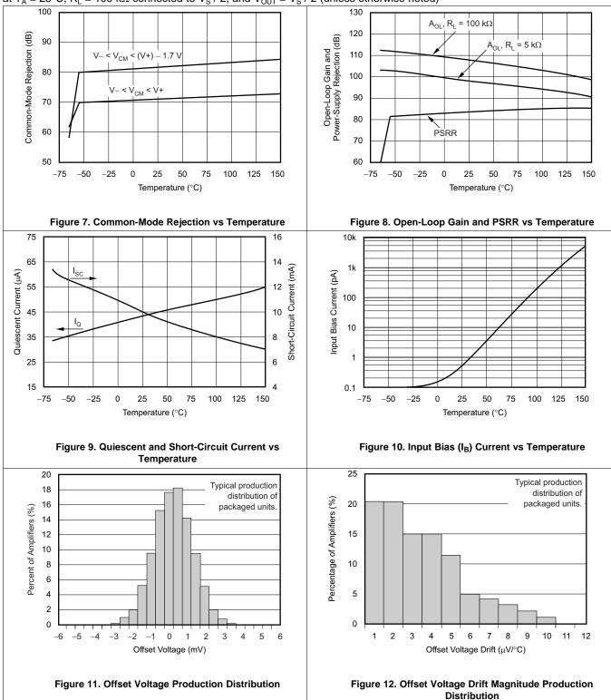
at  $T_A = 25^{\circ}$ C,  $R_L = 100 \text{ k}\Omega$  connected to  $V_S$  / 2, and  $V_{OUT} = V_S$  / 2 (unless otherwise noted)
