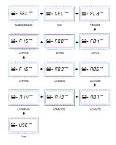
Note: If the controller supports 48V system voltage, the battery type will display LiFePO4 F15/F16 and Li(NiCoMn)O2 N13/N14.
