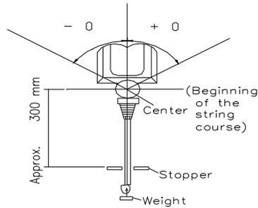
Bend in obverse at rate 20 time/min. and at an angle of  $\pm 60^{\circ}$ . Number of broken wire. Disconnection rate of the wire shall be 30% or less. and no abnormality on appearance.
