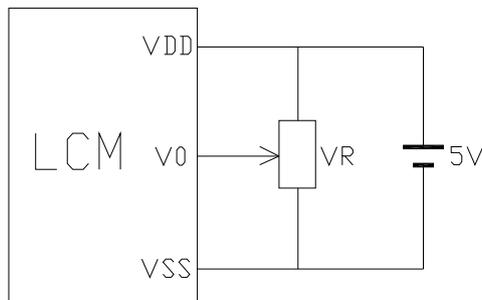
V<sub>DD</sub>-V<sub>0</sub>: LCD Driving voltage
