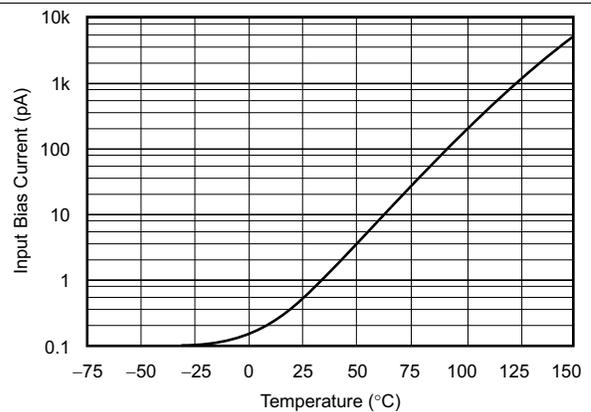
Figure 10. Input Bias ( $I_B$ ) Current vs Temperature
