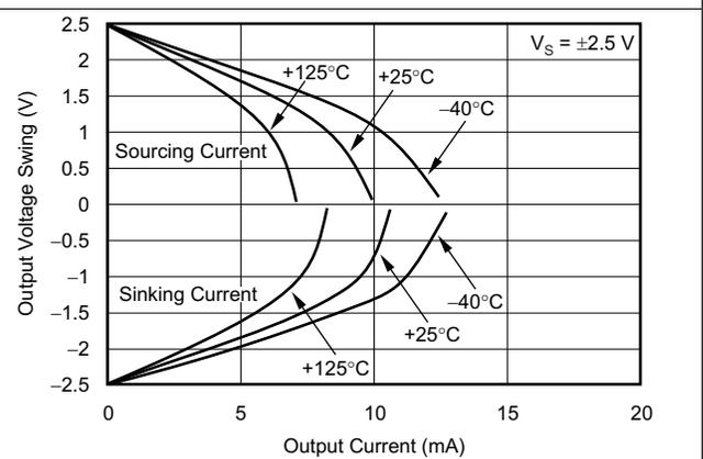
Figure 6. Output Voltage Swing vs Output Current
