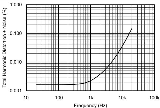
Figure 18. Total Harmonic Distortion + Noise vs Frequency
