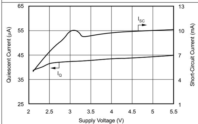
Figure 5. Quiescent and Short-Circuit Current vs Supply Voltage
