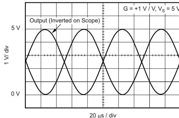
**Figure 24. OPA348 Features Rail-to-Rail Input and Output**
