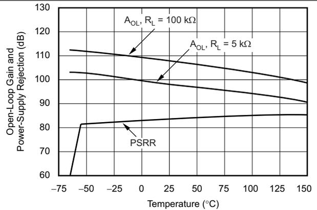
Figure 8. Open-Loop Gain and PSRR vs Temperature
