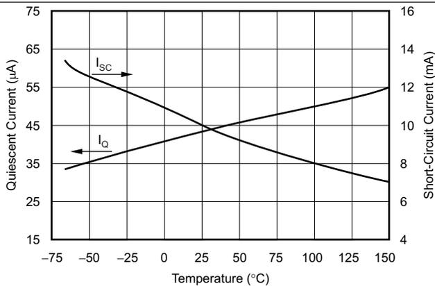
Figure 9. Quiescent and Short-Circuit Current vs Temperature
