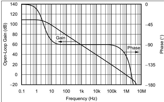
Figure 1. Open-Loop Gain and Phase vs Frequency
