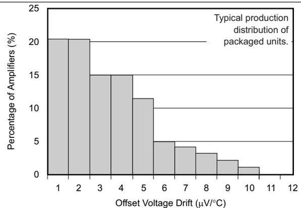
Figure 12. Offset Voltage Drift Magnitude Production Distribution
