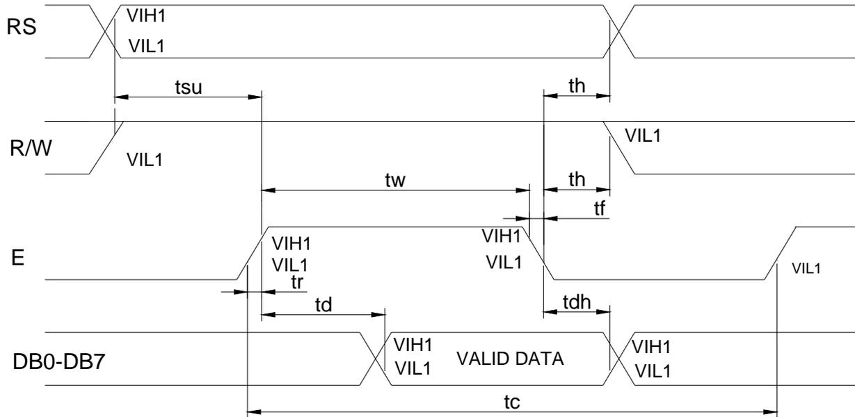
Write cycle ( $T_a=25^{\circ}C$ ,  $V_{DD}=5.0V$ )
