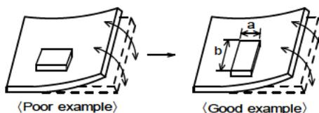
(2) Components location on PCB separation
