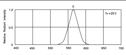
wavelength ヽ(nm) RELATIVE INTENSITY Vs. WAVELENGTH
