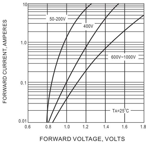
**Fig.3 FORWARD CHARACTERISTICS**
