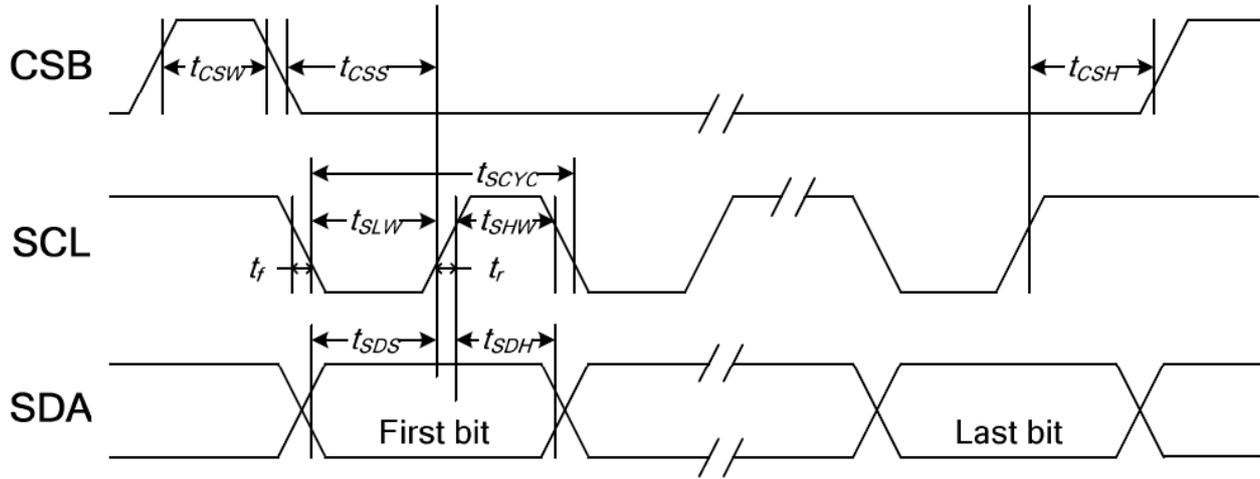
System Bus Timing for 3-Line Serial Interface
