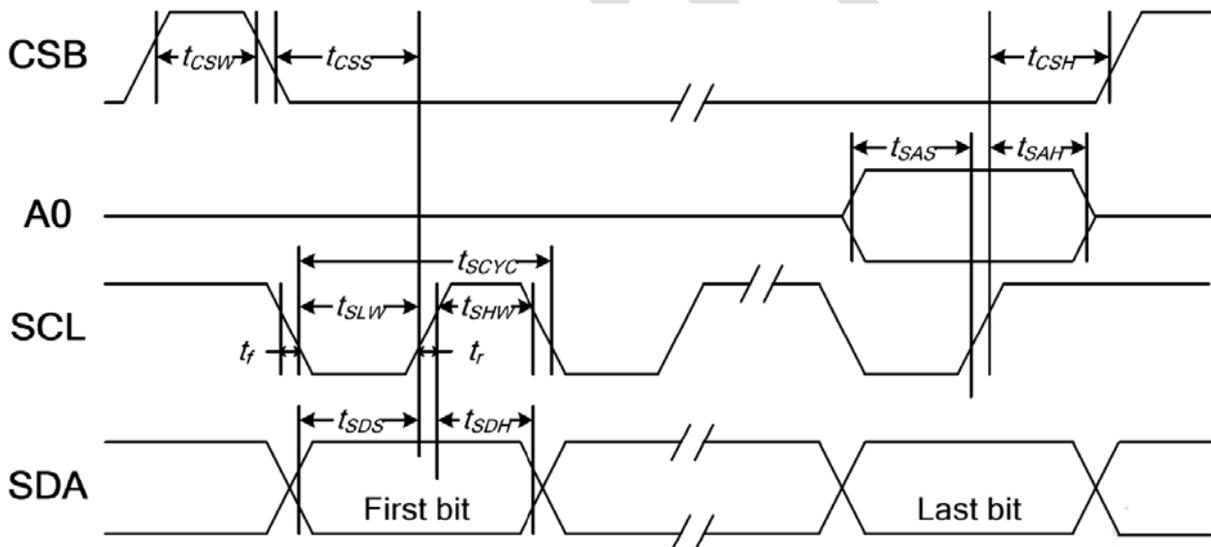
System Bus Timing for 4-Line Serial Interface
