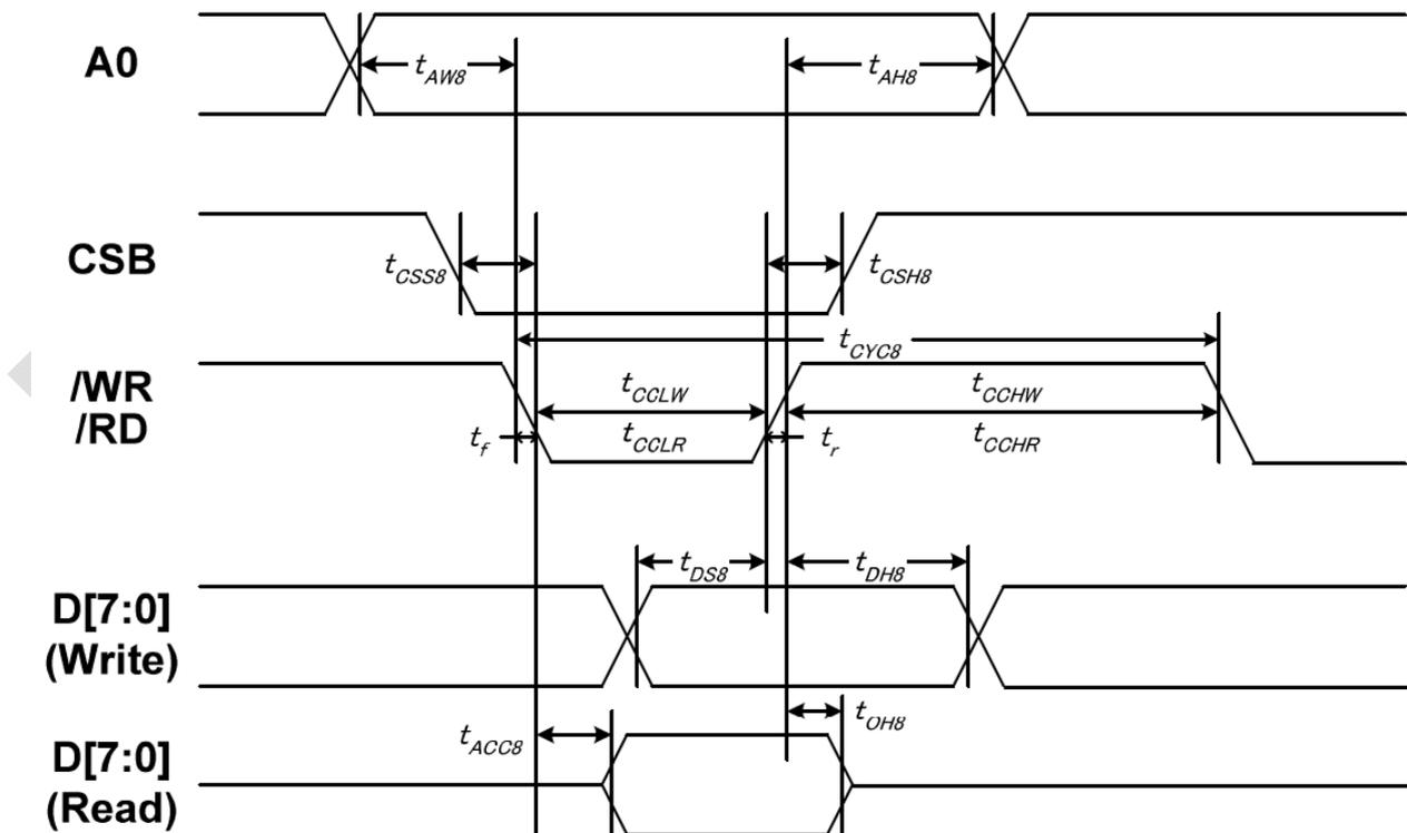
System Bus Timing for 8080 Series MPU
