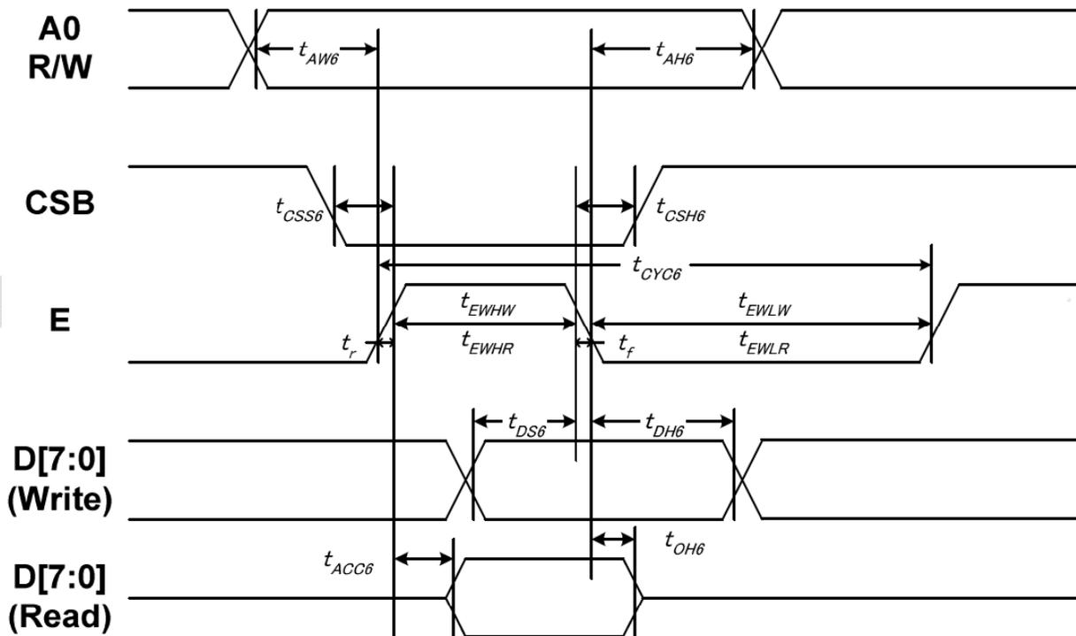
System Bus Timing for 6800 Series MPU
