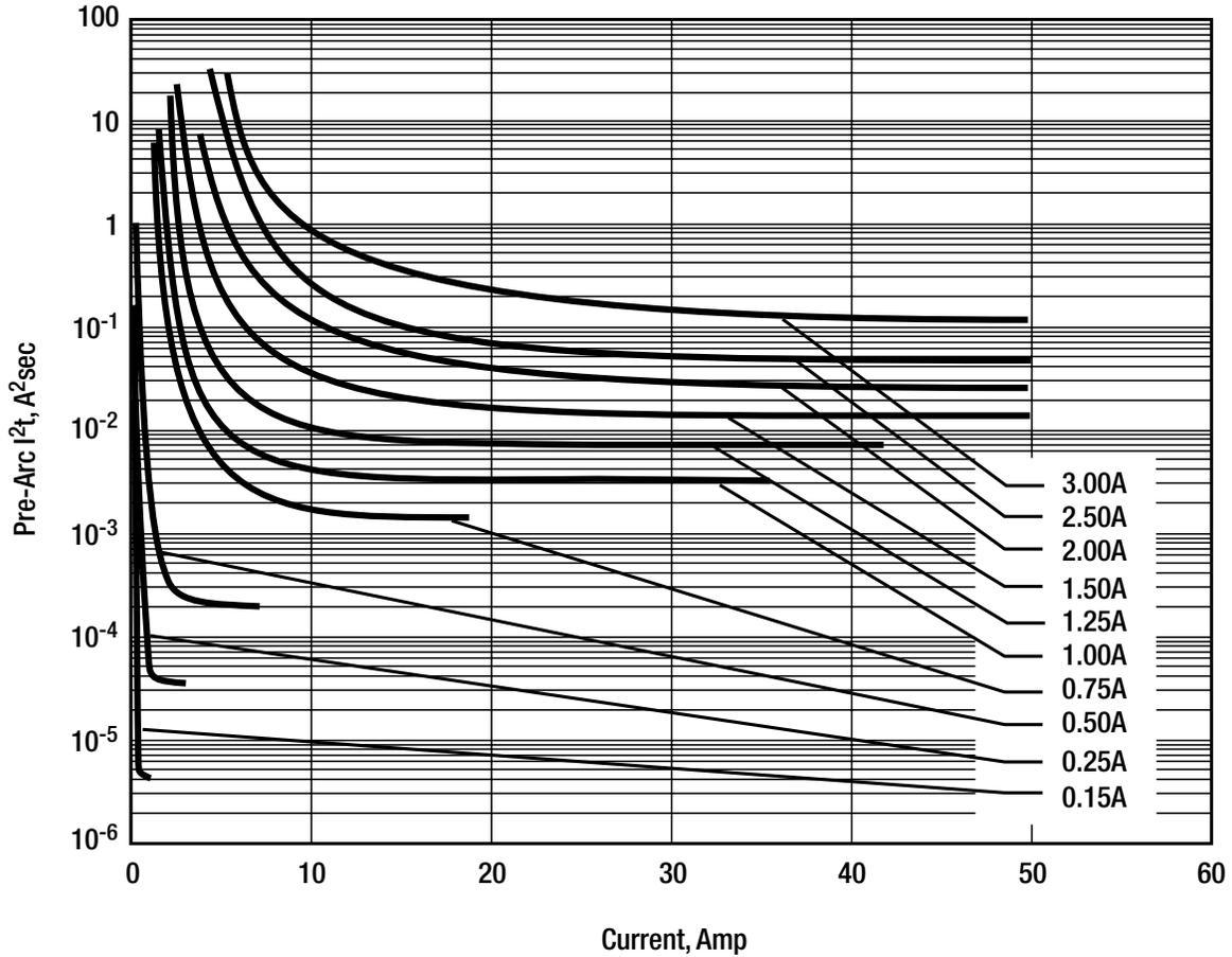
**FUSE PRE-ARC JOULE INTEGRALS VS. PRE-ARC TIME FOR TYPES F0805B AND F1206B (TYPICAL)**
