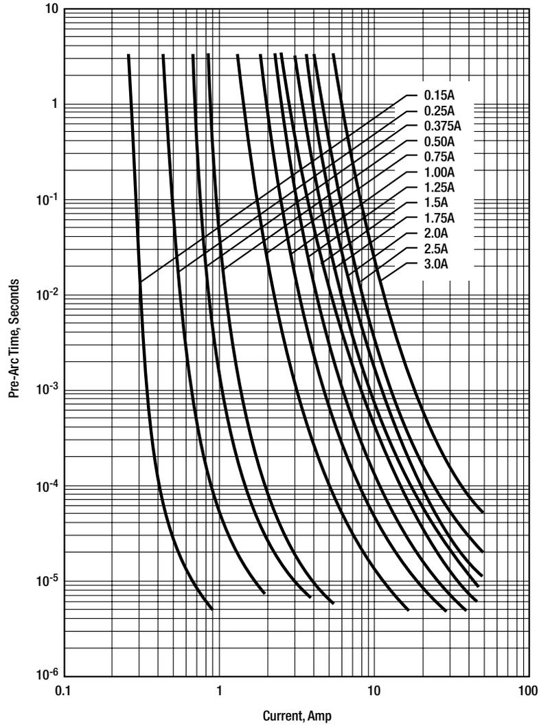
**FUSE PRE-ARC JOULE INTEGRALS VS. CURRENT TIME FOR TYPES F0805B AND F1206B (TYPICAL)**
