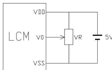
V<sub>DD</sub>~V<sub>0</sub>: LCD Driving voltage
