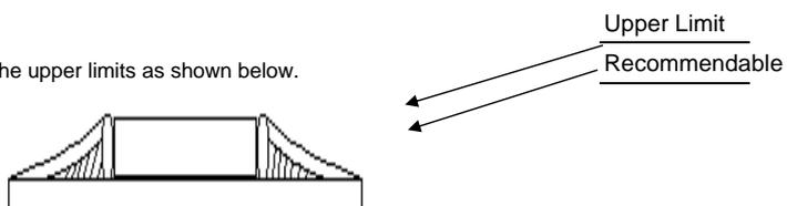
Accordingly increasing the solder volume, the mechanical stress to product is also increased. Exceeding solder volume may cause the failure of mechanical or electrical performance.
