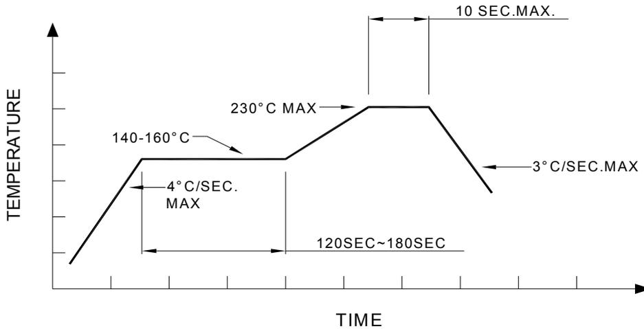
**Recommended Pb-free re-flow soldering profile:**
