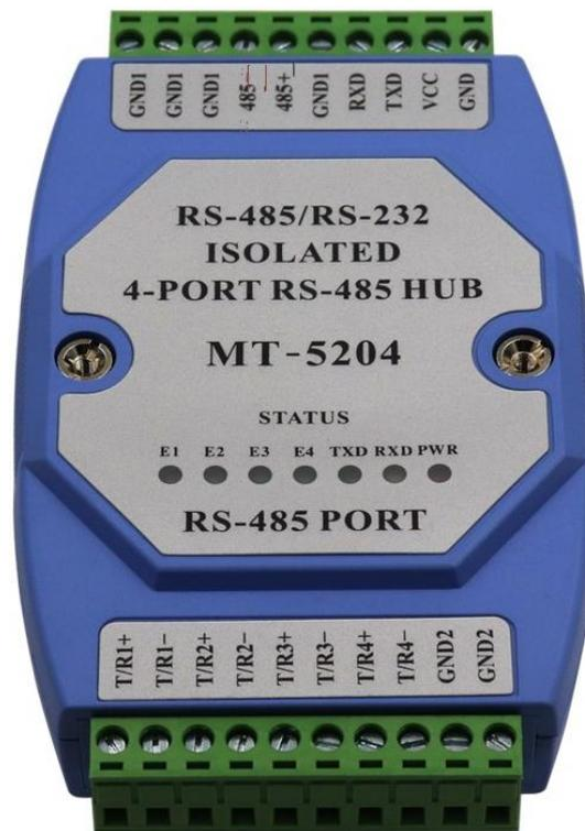
The hub provides a star RS485 bus connection, and each port has short-circuit and open-circuit protection. The optical isolation voltage is up to 2500V, and users can easily improve the RS485 bus structure, divide network segments, and improve communication reliability. When lightning strikes or equipment malfunctions occur, the faulty network segment will be isolated to ensure that other network segments
