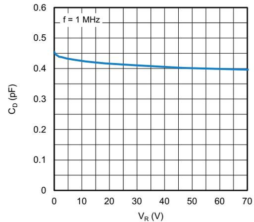
Fig. 3 - Typical Capacitance vs. Reverse Voltage
