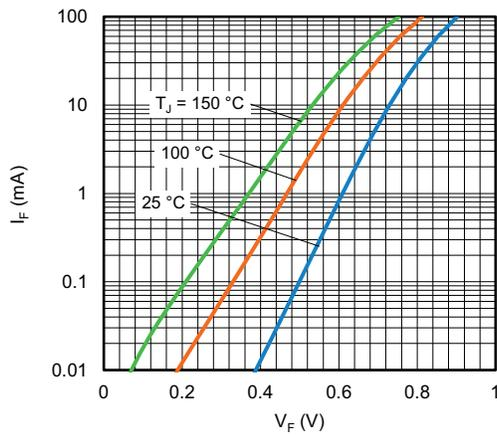
Fig. 1 - Typical Forward Current vs. Forward Voltage
