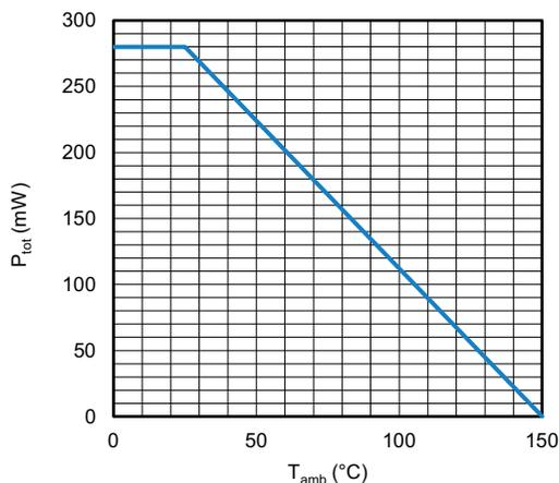
Fig. 2 - Admissible Power Dissipation vs. Ambient Temperature
