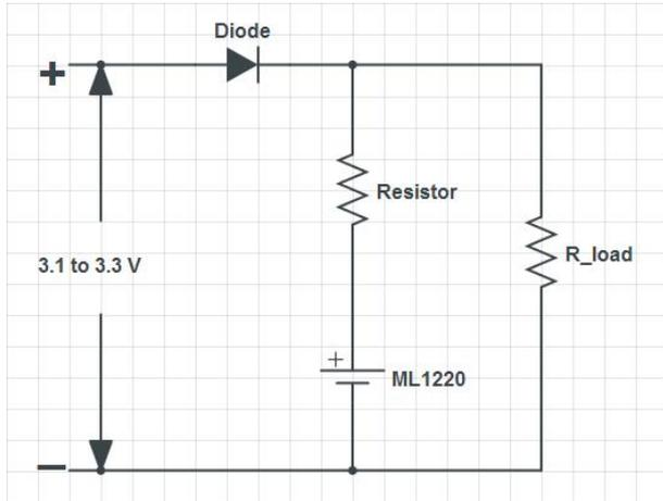
Figure 1 Recommended circuit of constant voltage charge with protective resistor
