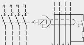
example below: 2 pole MCB + 2 pole RCD add-on block.
