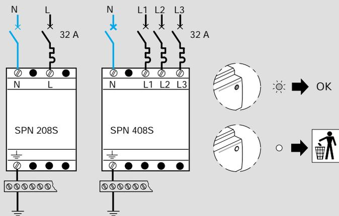
**Coordination :** between main SPD and secondary level SPDs, this coordination allows to reduce the protection level  $U_p$  to  $\leq 800$  V
