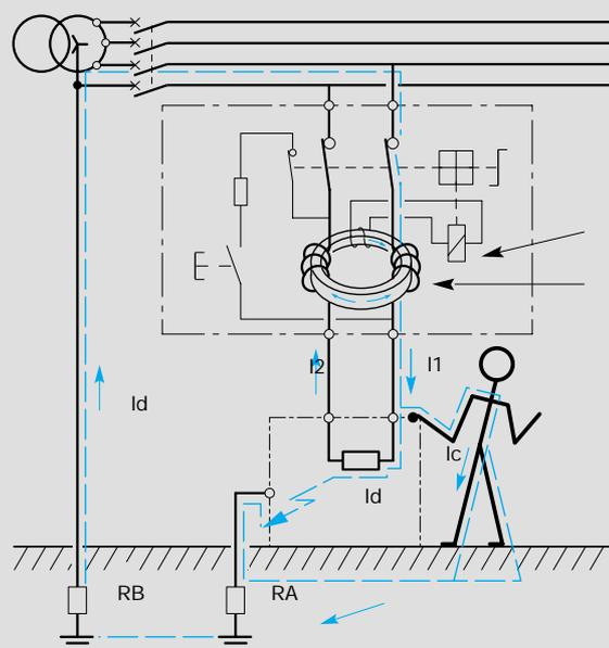
Current flowing through torroid in healthy circuit
