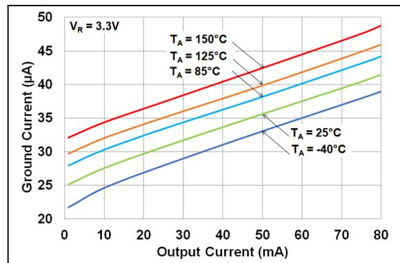
**FIGURE 2-12:** Ground Current vs. Output Current ( $V_R = 3.3\text{V}$ ).
