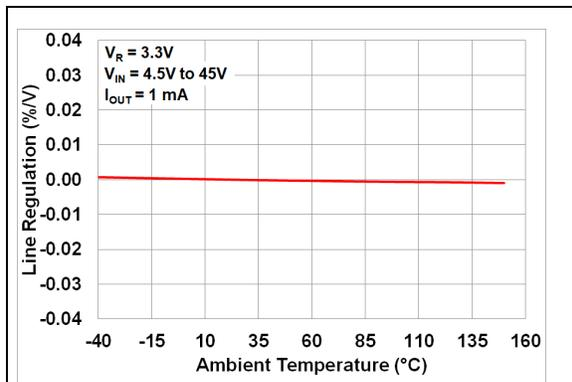
**FIGURE 2-8:** Line Regulation vs. Ambient Temperature ( $V_R = 3.3\text{V}$ ).
