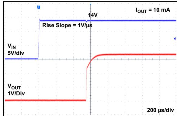
**FIGURE 2-22:** Start-up ( $V_R = 3.3\text{V}$ ).
