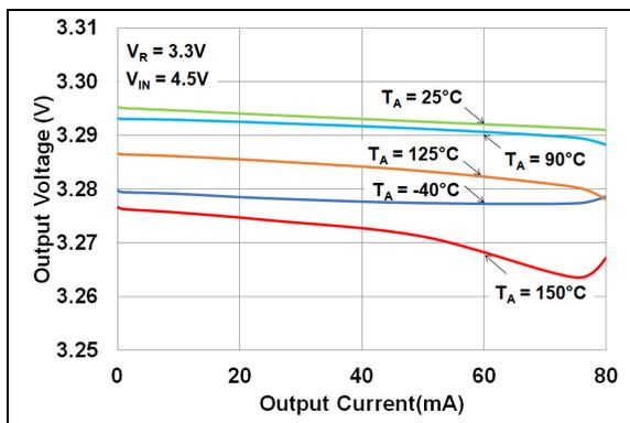
**FIGURE 2-3:** Output Voltage vs. Output Current ( $V_R = 3.3\text{V}$ ).
