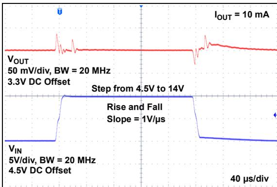
**FIGURE 2-20:** Line Step Response ( $V_R = 3.3\text{V}$ ).
