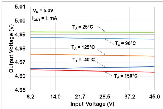
**FIGURE 2-2:** Output Voltage vs. Input Voltage ( $V_R = 5.0\text{V}$ ).
