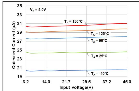
**FIGURE 2-11:** Quiescent Current vs. Input Voltage ( $V_R = 5.0\text{V}$ ).
