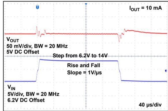
**FIGURE 2-21:** Line Step Response ( $V_R = 5.0\text{V}$ ).
